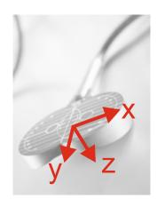
In all cases shown above, the view is onto the "active" side of the coil (i.e. the side attached to the subject's head)
